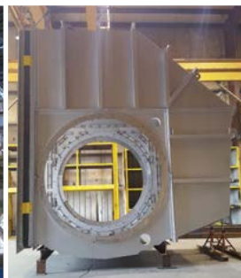
FS7EA exhaust plenum assembly.
